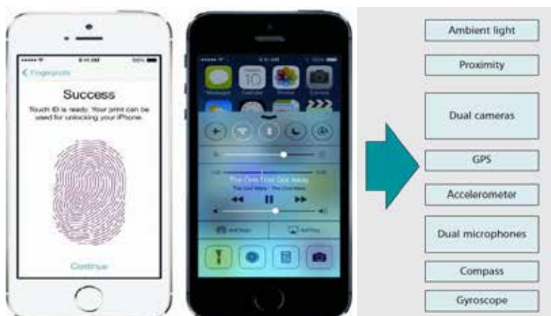
Figure 3: The sensors in iPhone 5s.
