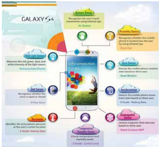
Figure 2: The sensors in Samsung Galaxy S4.
